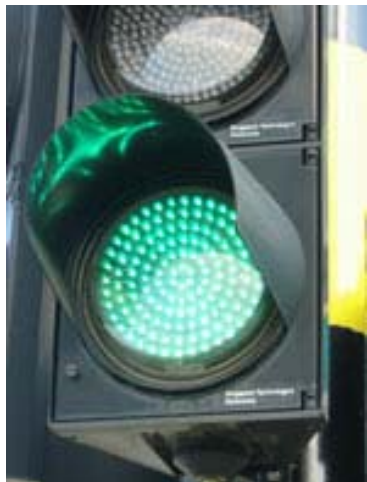
Retrofitted LED Stoplight
