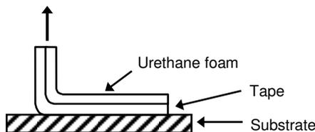
[Adhesive residue test method]
