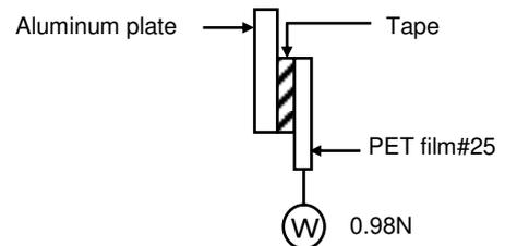
●Holding power -Aging(durability) at each condition after applying
