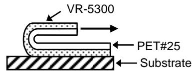
● 180 degree peeling strength for each temperature
